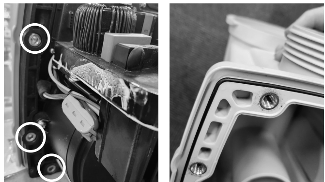
Step 5: Remove all 8 x bolts with an Allen key. (Be careful there is a small O-ring that seals around the top on the body)
