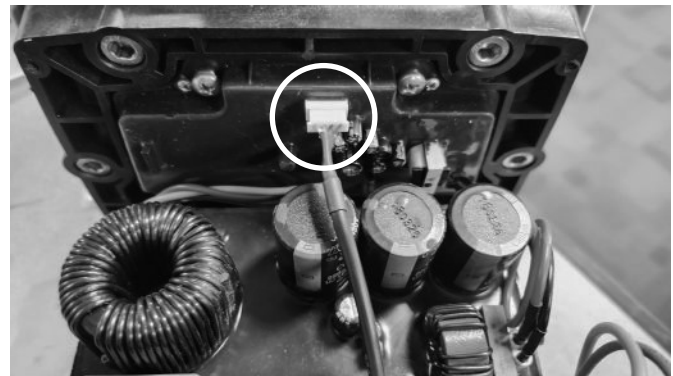
Step 3: Disconnect the signal wire for the display.
