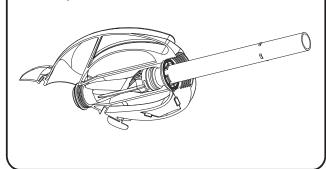
(f) Slide the THRUST WASHER over the INNER EXTENSION PIPE. The flat side (widest diameter) of the THRUST WASHER should be face down.
