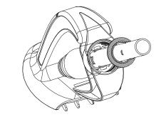
(g) Place the OUTER EXTENSION PIPE over the INNER EXTENSION PIPE.
