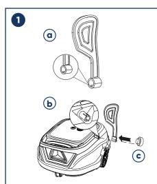
Insert the flipper (a) into the cleaner, ensuring that its notch is aligned with the groove (b) on the right side of the cylinder. It should click into place. Push rubber cap (c) into round opening on (b).
