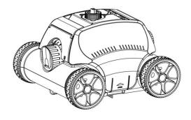
Hold Both sides of the top cover near the clips and pull out + lower the top cover over the chassis until it clips into place.
