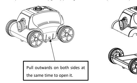
b. Lift the filter tray off the chassis
