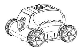
Hold Both sides of the top cover near the clips and gently pull clips outward + lower the top cover over the chassis until it clips into place.
