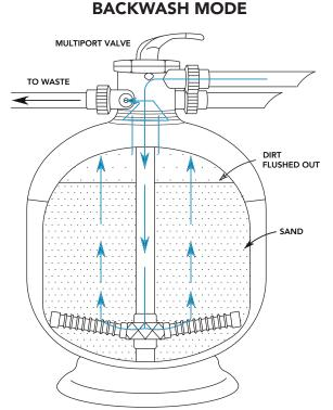
glass on the backwash filter returns clear, turn the system off again. Switch the handle to "Rinse" and restart the pump for 30-60 seconds until the sight glass clears once more. Turn off the system again and switch back to "Filter" to resume normal pump and filter system operation.
