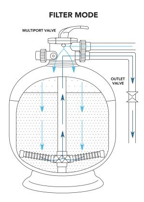
The filter employs special filter media to eliminate dirt particles from the pool water. This media is loaded into the filter tank and acts as a permanent dirt removal system. When the control valve is set to the filter position, the pool water, which contains contaminated particles, is pumped through your piping system, and automatically directed through the filter's Multiport valve. As the water passes through the filter, dirt particles are trapped by the media and filtered out.
