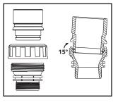
Wait 24 hours before running the filter to allow the Glue to set correctly. (consult the PVC Glue directions for use)
