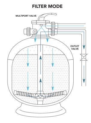
The filter employs special filter media to eliminate dirt particles from the pool water. This media is loaded into the filter tank and acts as a permanent dirt removal system. When the control valve is set to the filter position, the pool water, which contains contaminated particles, is pumped through your piping system, and automatically directed through the filter's Multiport valve. As the water passes through the filter, dirt particles are trapped by the media and filtered out.
