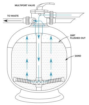
glass on the backwash filter returns clear, turn the system off again. Switch the handle to "Rinse" and restart the pump for 30-60 seconds until the sight glass clears once more. Turn off the system again and switch back to "Filter" to resume normal pump and filter system operation.
