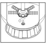
**IMPORTANT: MAKE SURE EACH LATERAL IS NOT DAMAGED OR CRACKED.** You will not be able to successfully install the filter if a lateral is cracked as any media in the filter will return to the pool. Contact Hy-Clor for assistance.
