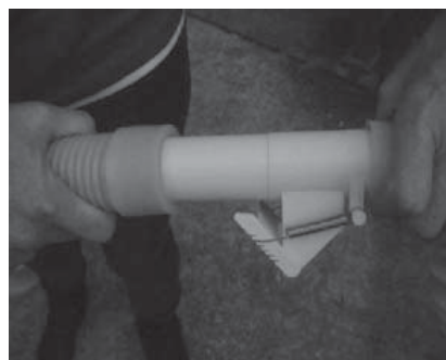
Push hose firmly onto speed control valve
