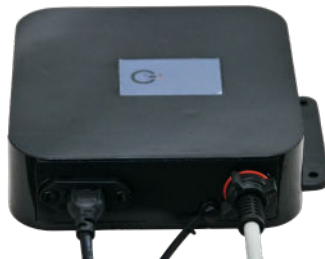
4.2 Insert the end of the floating cable into the socket. Be careful with the direction of the plug.
