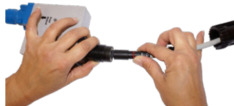
4.3 Insert the end of the floating cable from the transformer into the black "POWER" socket. Be careful with the direction of the plug.
