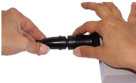
4.4 Slide the cap to contact the plug of the floating swivel union.
