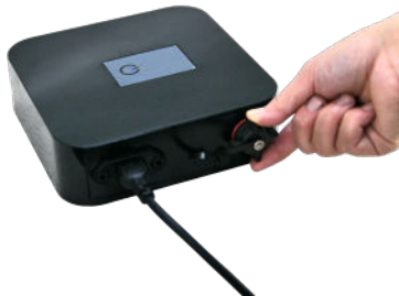
4.1 Unscrew the cap next to the switch.
